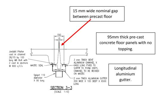
Figure 2.2.4: section of aluminium guttering in place.
