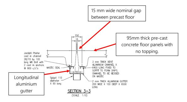
Image below shows a section of aluminium guttering in place.
