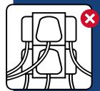
**DON'T** overload plug sockets - too many items can draw power from the one socket and can overheat. An extension lead or adaptor will have a limit to how many amps it can take.
